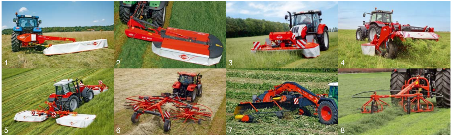
1. Rear disc mowers 2. Rear drum mowers 3. Front-mounted mowers and mower conditioners 4. Rear disc mower conditioners 5. Triple gang mowers and mower conditioners 6. Gyrorakes 7. Belt mergers 8. Tedder-rake combinations
